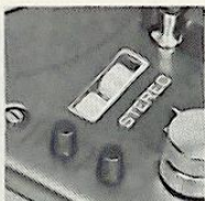
1. The bass can be continuously increased and treble can be continuously decreased by means of individual controls.
