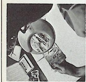
Optical inspection of the printed circuits.
