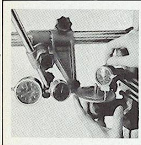
All parts are inspected on arrival at the factory. This picture shows the checking of the turntables for accuracy.
