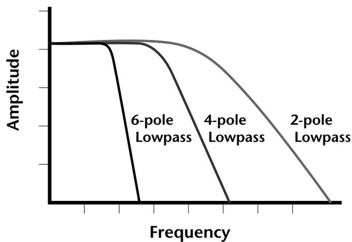
Using a filter, we have a way to control the harmonic content of a sound. As it turns out, even a simple low-pass filter can simulate the response of many natural sounds.
