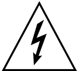
*This symbol is intended to alert you to the presence of uninsulated dangerous voltage within the product's enclosure that may be of sufficient magnitude to constitute a risk of electric shock to persons.*
