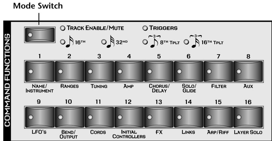
The mode switch is normally used to select between Triggers and Track Select/Mute. In Sequencer Grid Edit, the mode switch is used to select step resolution.
