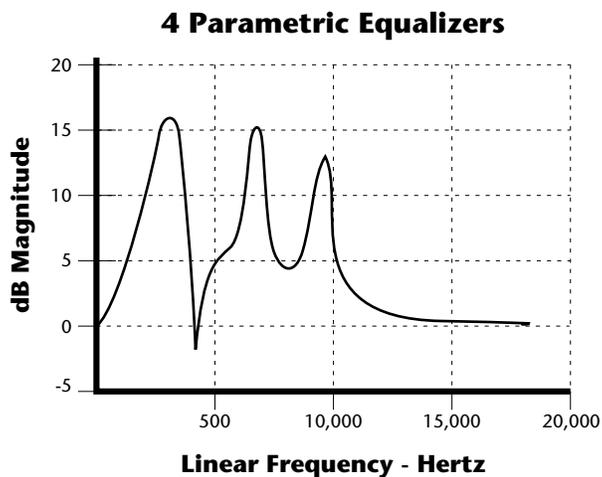
Many natural instruments have complex resonances which are based on their soundboard or tube size. The resonance shown above would be impossible to create using a normal synthesizer filter.
