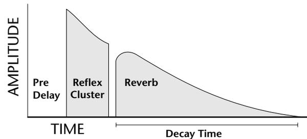
After an initial pre-delay period, the echoes from the closest walls or ceiling are heard. These first echoes, or the early reflection cluster, vary greatly depending on the type of room. Roughly 20 milliseconds after the early reflection cluster, the actual reverberation begins and decays according to the time set by the Decay Time parameter.
