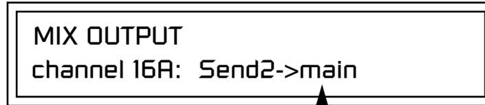
*Indicates that the dry signal is routed to the Main output jacks.*
