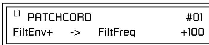
This setup connects the Filter Envelope Generator to the Filter Cutoff as shown in the following diagram.
