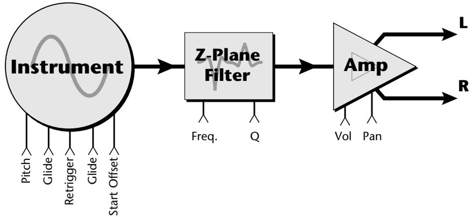
To understand how a filter works, we need to understand what makes up a sound wave. A sine wave is the simplest form of sound wave. Any waveform, except a sine wave, can be analyzed as a mix of sine waves at specific frequencies and amplitudes.
