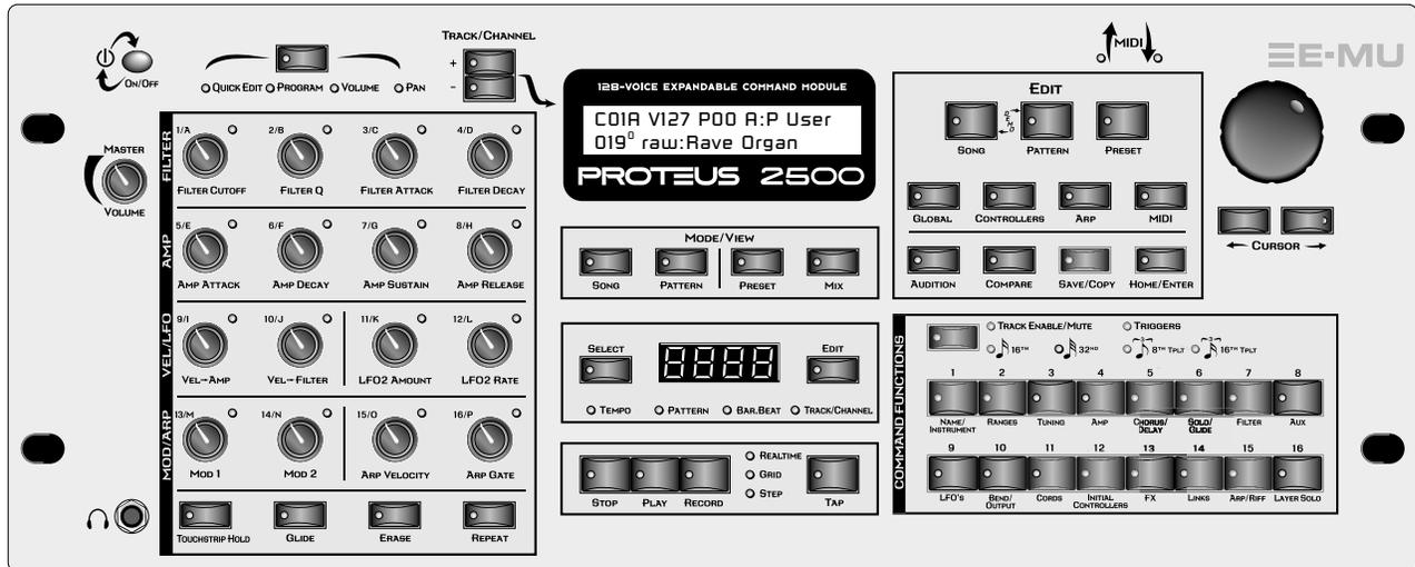
The Proteus 2500 front panel contains an LCD screen, 49 buttons, and 16 real-time controller knobs. Functions are grouped logically and the controls are arranged for ease of use.
