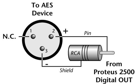
If you use an adapter cable to connect the S/PDIF digital audio output to AES gear, make sure to use high quality, low capacitance cable.
