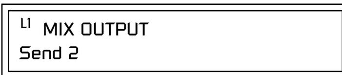
Why have a Send 4 routing at all if it only goes to the Main output? The answer lies in the dual function of the Sends. Sends can be used either as *Effect Sends* or as *External Output* routing busses. Send 4 is only used as an effect send, while Sends 2 and 3 can be used as effect sends or external routing busses.
