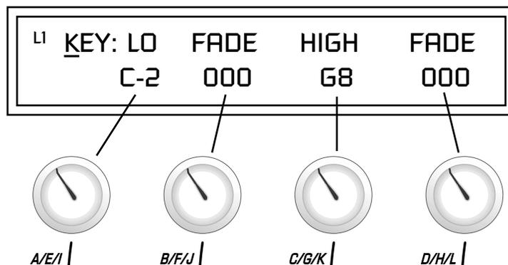
To move through menus horizontally, use the Data Entry Control (the page’s title field is the default cursor position). To move through menus vertically (preset layers), press the left cursor to get to the layer field, then change layers with the Data Entry Control.
