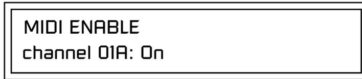
Because the MIDI Enable function only makes sense if you are in Multi mode, Virtuoso 2000 disables this feature when in Omni or Poly mode.
