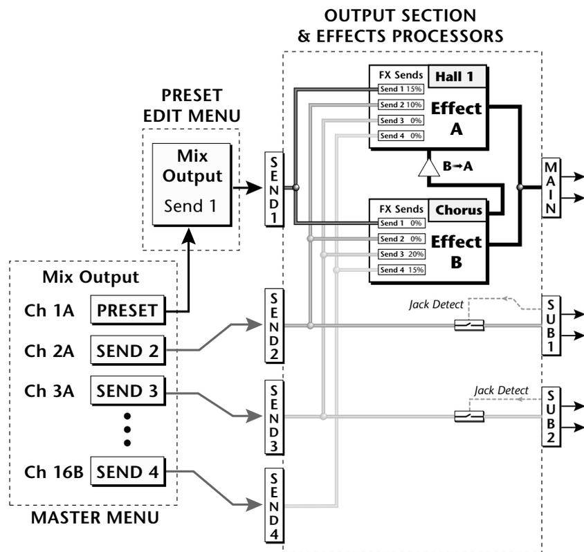
Individual layers or entire MIDI channels can be routed to any of the four busses.
