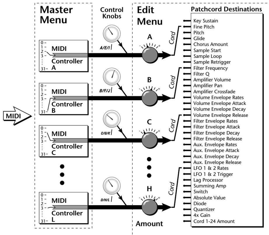
MIDI A-L are internal connections which simultaneously carry front panel controller knob data and MIDI continuous controller data.
