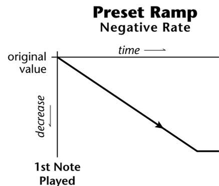
The preset ramp instantly resets when all notes have been released and the next *first key* on the MIDI channel is pressed. The Ramp Rate polarity (+ or -) determines if the ramp will be positive or negative going. The value of the ramp rate sets the increment. Large values produce fast ramps and small values produce slow ramps. Multiple inputs can be connected to the ramp rate (just like all the other destinations in Virtuoso 2000).
