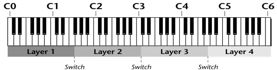
Just assign the low and high key range for each of the four layers with Fade set to zero. Set the Low and High Keys so they don't overlap other layers.
