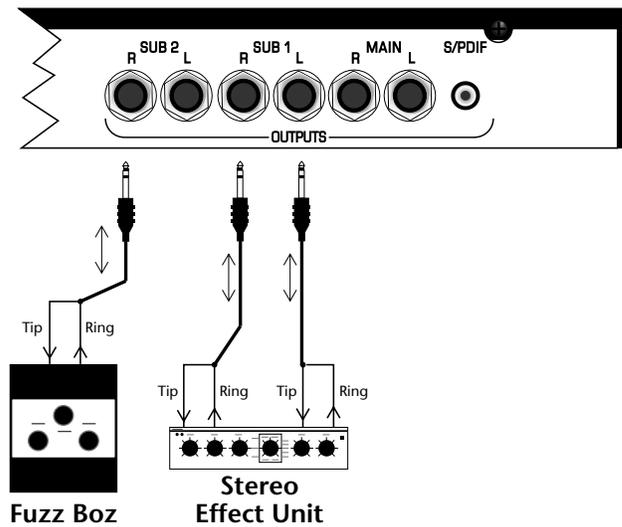
Using the submix outputs and returns, specific presets can be routed through your favorite effects without using up precious mixer channels.
