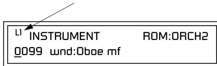
When "All Layers" (A) is selected, the existing parameter value for any field will be displayed if all layers are equal. If the layer parameter values are NOT equal, the value of Layer 1 will be displayed with flashing characters. If you move the Data Entry Control all values will be equal to this new value and the parameter value will no longer flash.
