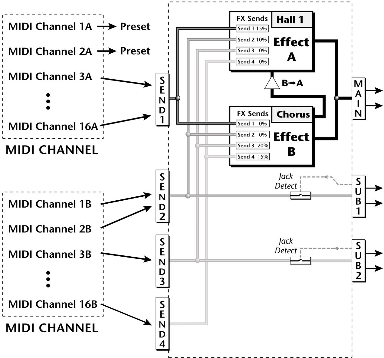
Sends 2 and 3 can be routed to the effects processors or to rear panel submix jacks. When a plug is inserted into a Submix jack, the dry portion of the Send is disconnected from the effects processor and is routed **directly** to the Submix output jacks.
