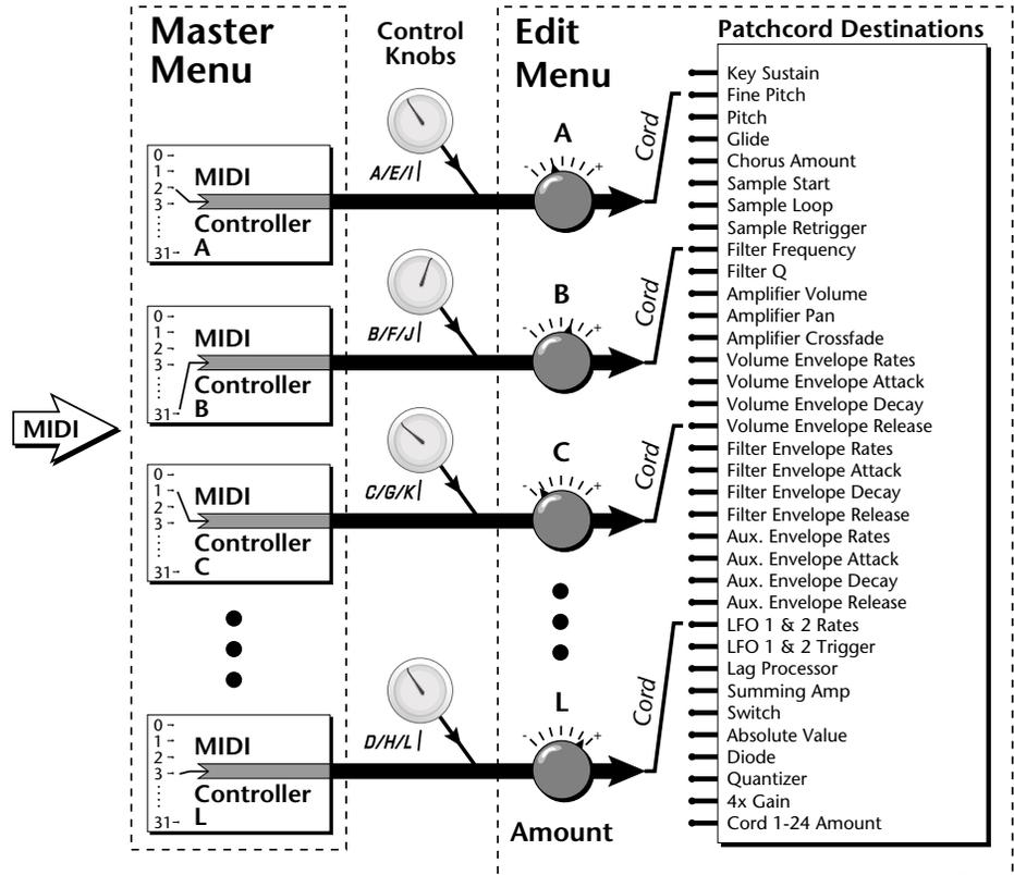
External MIDI controller numbers are assigned to the Letters A-L in the Master menu. The Initial Controller Amount value is sent to the PatchCord destination when the Preset is first selected. If you move the Control Knob, then that value replaces the initial value. If MIDI controller data is received it will similarly replace the knob or initial setting.
