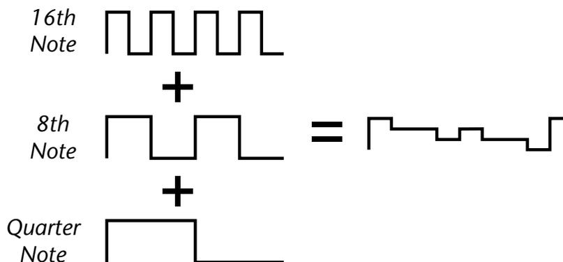
Adding multiple clocks with unequal amounts produces complex repeating patterns.
