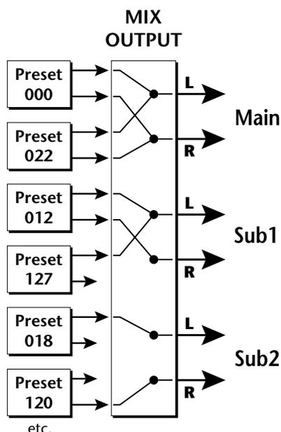
Each preset can be routed to one (and only one) set of stereo outputs. A preset can be routed to a single output using the pan control.
