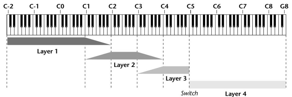
With a High Fade value of zero (as in layer 3 of the diagram), the layer simply switches off at the high key.
