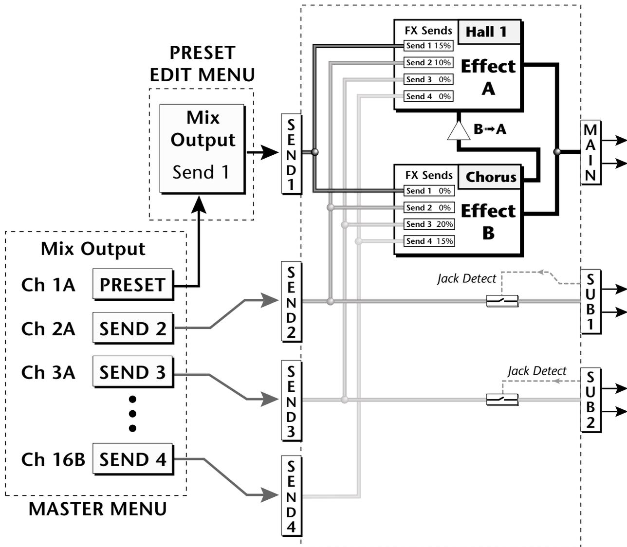
The Mix Output setting in the Master Menu determines if the Preset's Mix Output routing will be used. This allows the Sends to be programmed by either **MIDI Channel** or by **Preset**, whichever you prefer.
