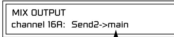
Indicates that the dry signal is routed to the Main output jacks.
