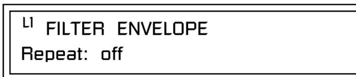
3. Move the cursor underneath the on/off field, then turn the data entry control clockwise so that Repeat is On.
