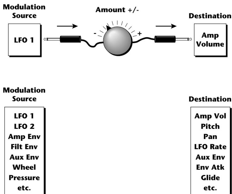
Each patch has an amount field which determines how much modulation is applied to the destination. The modulation amount can be positive or negative. Negative values invert the input. The amount value range is from -100 to +100.
