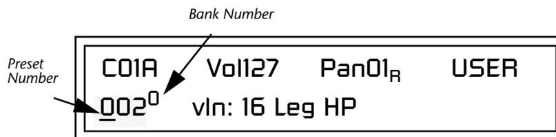
Using the screen above as an example, the superscripted number 0 in the second line of the display identifies the current bank number.
