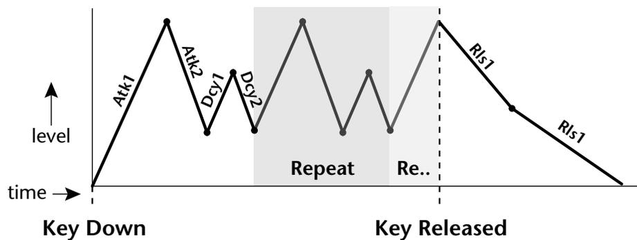
The diagram above show how the looping envelopes work. When the key is pressed the envelope goes through its regular Attack 1, Attack 2, Decay 1 and Decay 2 stages. In non-looping mode, the envelope would hold at the end of the Decay 2 stage until the key was released. In looping mode however, it jumps back to the Attack 1 stage and repeats the first four stages. It continues to loop through these four stages until the key is released where it immediately jumps to the Release 1 stage.
