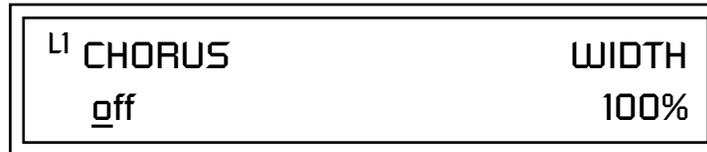
The first field in this screen turns Chorus On or Off and allows you to adjust the amount of detuning (1 to 100%). The *Width* parameter controls the stereo spread. 0% reduces the chorus to mono and 100% provides the most stereo separation.
