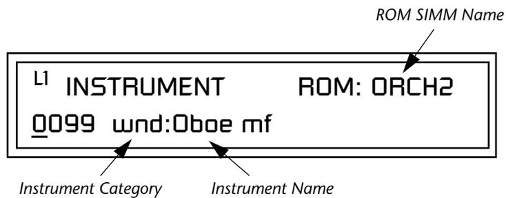
To select an instrument for the selected layer(s), move the cursor to the bottom line of the display and change the instrument using the Data Entry Control.
