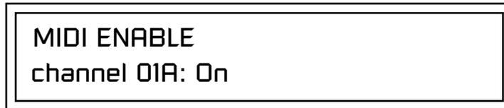
Because the MIDI Enable function only makes sense if you are in Multi mode, Virtuoso 2000 disables this feature when in Omni or Poly mode.
