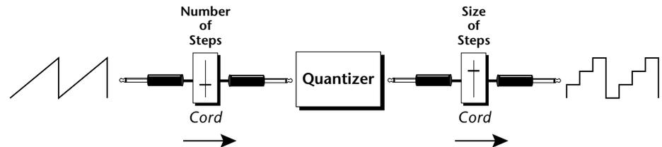
The input PatchCord amount controls how many steps will be generated. With a sawtooth wave (LFO+) feeding the input and the PatchCord amount set to 100%, sixteen steps are generated. The output PatchCord amount controls the size (or interval) of the steps.
