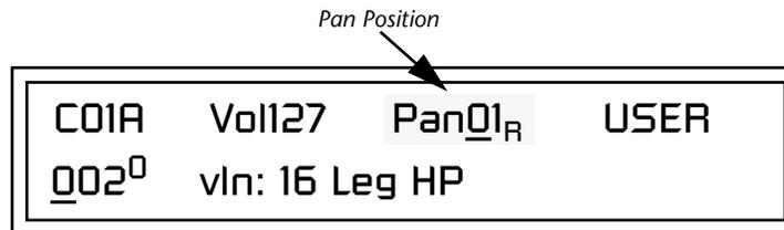
**Note:** Pan settings in the preset ADD algebraically with the Channel Pan setting. Therefore, if the pan setting in the preset were set to “63R,” moving the Channel Pan setting full left would return the sound to the center position.
