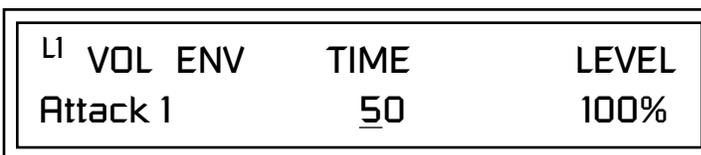
3. Increase the Attack 1 time value and play a note. The attack controls the time it takes for the sound to reach the Attack level when a key is pressed and held.
