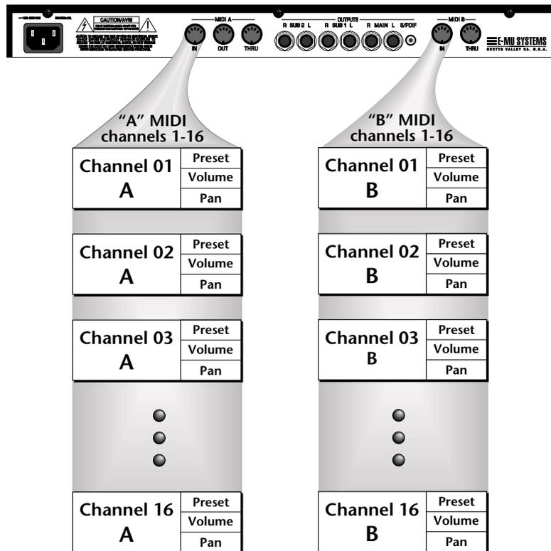
Virtuoso 2000 has two MIDI inputs with 16 MIDI channels each. Each of the 32 MIDI channels can be assigned to play a specific preset with unique volume and pan settings.
