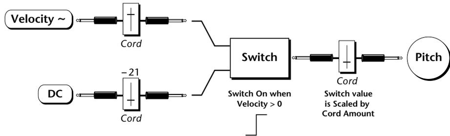
Connect the DC level to the input of the switch along with the velocity value. Note that more than one modulation source can be applied to the input of a processor.
