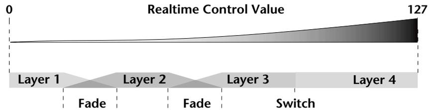
After the Ranges and Fades have been adjusted for each layer in the Real-time Crossfade screen, you must assign a real-time controller to RTXfade (Real-time Crossfade) on each Layer in the PatchCord screen. Set the PatchCord Amounts to +100.
