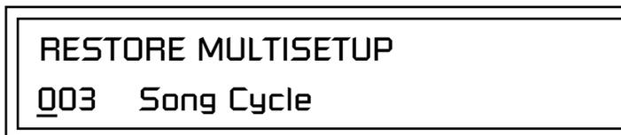
Multisetups can also be restored (selected) via MIDI Bank and Program change commands. Select: cc00 = 80, cc32 = 00, (dec) then send a Program Change command corresponding to the Multisetup you wish to select.
