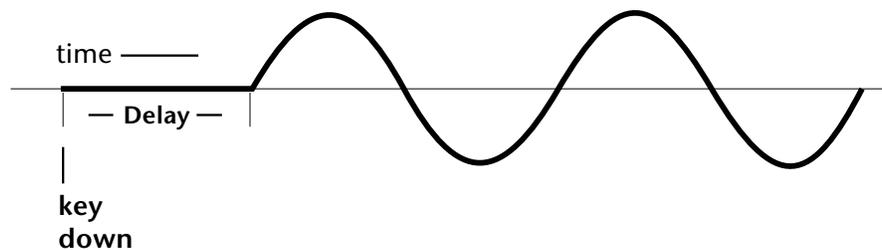
All Delay values equal to or greater than zero specify absolute time rates from 0 to 127. Values less than zero specify Tempo-based mode. Refer to the previous table for times and tempo-based rates.
