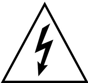
*This symbol is intended to alert you to the presence of uninsulated dangerous voltage within the product's enclosure that may be of sufficient magnitude to constitute a risk of electric shock to persons.*
