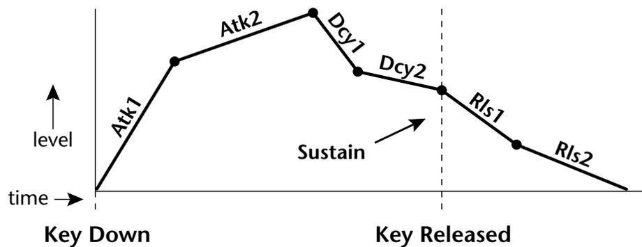
On the Volume Envelope, levels can only be set to positive values. The value range is from 0 to +100.
