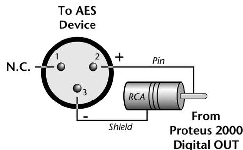
If you use an adapter cable to connect the S/PDIF digital audio output to AES gear, make sure to use high quality, low capacitance cable.
