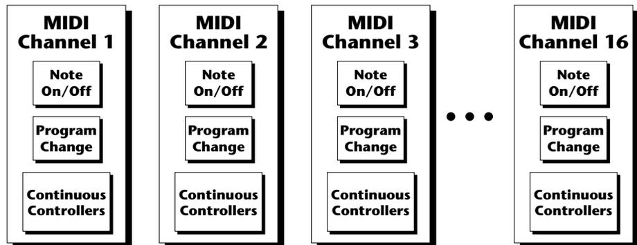
Any MIDI controller can be routed to any modulation destination. First, you have to know which controller numbers your keyboard transmits. Most modern MIDI keyboards let you select a controller number for each control on the keyboard. For example, it may let you select a number from 0-31 for the data slider. The realtime controller numbers that the keyboard transmits must match the numbers Virtuoso 2000 is receiving, otherwise nothing will happen when you move the controls.
